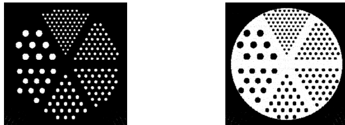
Figure 6. Ideal images reconstructed with complete projection data. (left: hot-rod phantom, right: cold-rod phantom)
